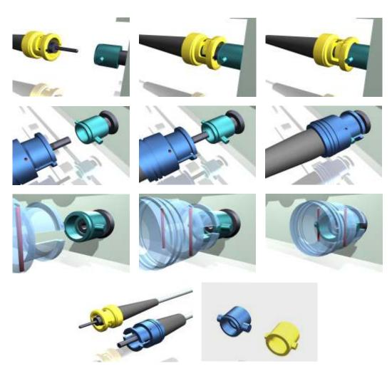
Frames from an animation illustrate the difference and incompatibility between two connectors. Even though the two connectors look similar, the animation demonstrates that they work differently. Transparency shows the inner workings and a final side by side view emphasizes differences between the two.
